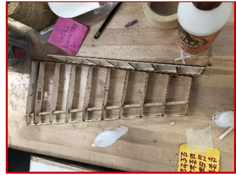
Fig. 5.1.5.1.4 Rudder During Assembly
