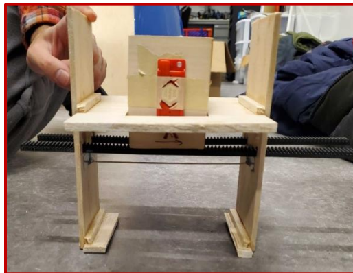
Fig. 7.1.1.3.2 Drop Test Rig, with Package Prototype, Racks, and Rubber Band Shown
