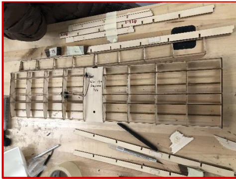
Fig. 5.1.5.1.3 Horizontal Stabilizer During Assembly
